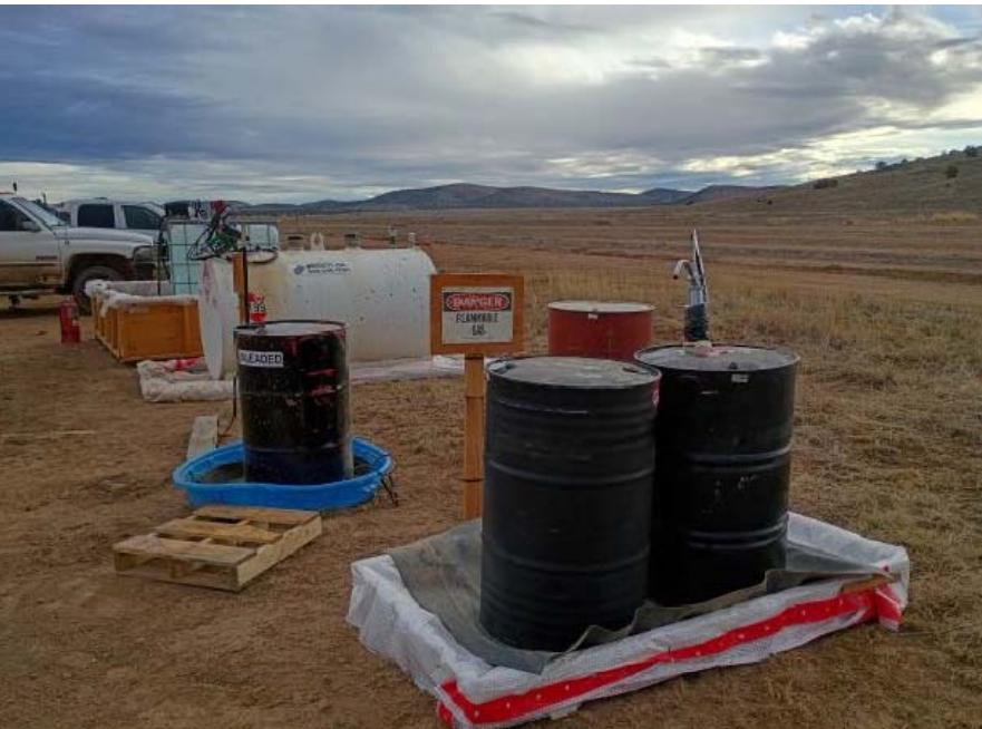
A photograph showing fuel storage tanks in a secondary containment system. There are several large black metal drums arranged on a white and red containment berm. One of the drums has a sign that reads "DANGER FLAMMABLE LIQUID". In the background, there is a white pickup truck and a white storage tank. The ground is dirt and there are mountains in the distance under a cloudy sky.                                                                                 |
