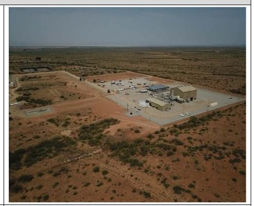
Location: Dragoon Compressor Station Description: Suction pipelines tie in yard after painting, grading, gravel and security fencing completed.
